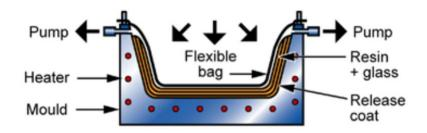
Vacuum bagging largely follows the same principle as wet lay-up. The difference is on the curing process. The curing is made this time in a vacuum bag.[6] Mold may be heated if the process is used to make finished goods. Compare to the wet lay-up, this process allows a Higher fiber contents, a lower porosity, and a better process control. This is used for large boat hulls, aircraft structures.
