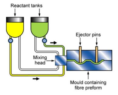
This method allows high-tech composite pieces.[6] The main advantages of this process is the precision and the surface quality of the molded pieces. A dry preform fiber pieces is introducing in the print of the mold, then with high pressure the resin is injected in the mold. The mold stay closed until the curing is finish and then the piece is ejected. However, this process is really expensive and only use for high quality composite.
