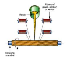
This process involves winding filaments under tension over a rotating mandrel.[6] The fibers are impregnated in a bath with resin as they are wound onto the mandrel. Further, the method allows for precise control of the direction of the fibers in the product. This process is usually use for pipes or another cylindrical object.
