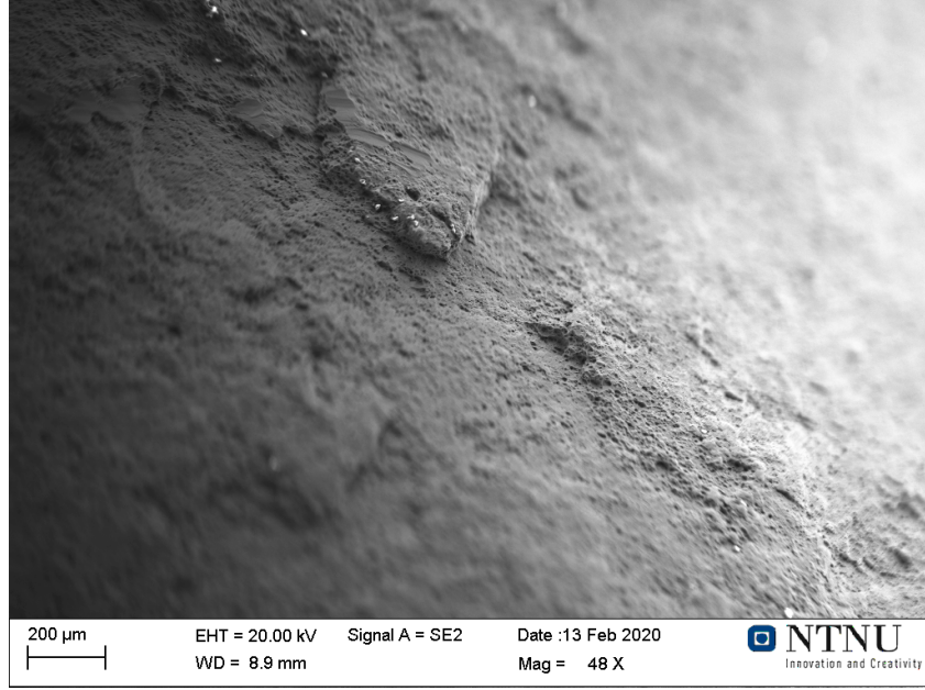
Figure 4: 120 \mu m aperture, 10 mm working distance, high current off. Theoretical depth of field: 0.079 mm
